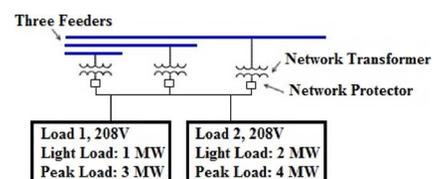
Fig. 4. Typical configuration of an isolated spot network.
