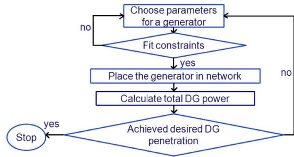
Fig. 5. Allocation algorithm for nondeterministic DG units.
